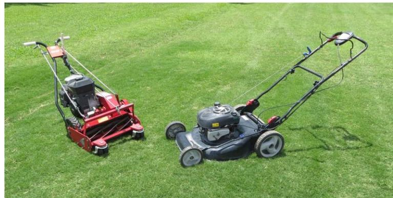
**Reel-type mower (left), and rotary mower (right)**
