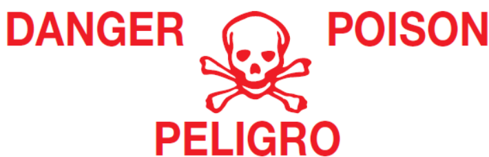
Figure 2. The “DANGER – POISON” Signal Words are always accompanied by the skull and cross-bones, which tells the user that this product is highly toxic by any route of entry.
