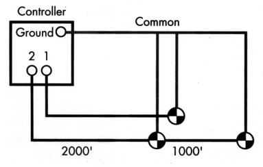
2. Calculate the "equivalent circuit length" for each valve circuit.
