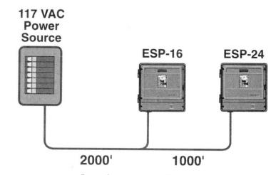
5. Select a power wire size from Rain Bird chart that has an F factor *equal to or less than* the calculated F factor.
