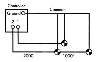
3. From the Rain Bird wire sizing chart, select the common and control wire sizes for the circuit with the highest equivalent circuit length (the "worst case" circuit).
