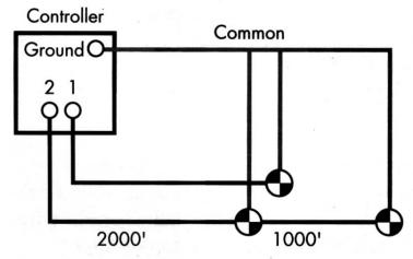
4. Having the common wire established, use the wire sizing chart to determine the control wire size for each of the remaining valve circuits on the controller.
