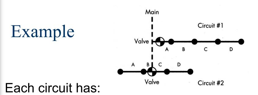
4 medium-sized rotor pop-up sprinklers, that throw 47 ft radius at 55 psi and require 9.8 gpm each.
