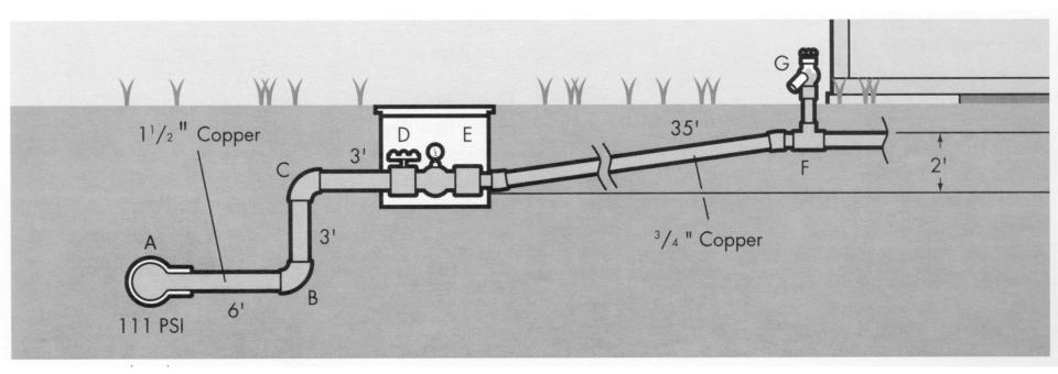
If water flow is 20 gpm, what is the dynamic water pressure, in psi, at points: B?
