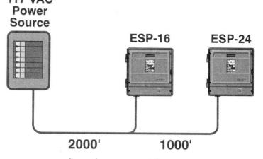
2. Determine the maximum allowable voltage drop along the wires from the power source to the controllers.
