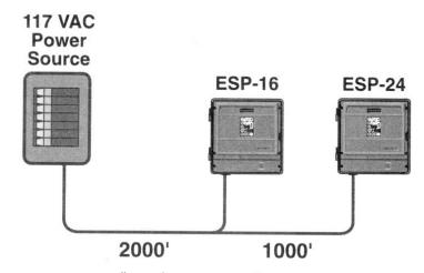
3. Calculate the equivalent circuit length for the power wire and controller(s).
