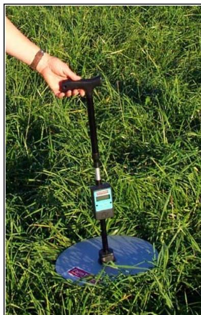
**Fig. 3.** To use the rising plate meter to measure pasture height, place the plate on the pasture canopy and, holding the shaft vertically, push it down to the ground. This makes the plate rise up the shaft, moving the counter that measures the height of the plate above the ground.
