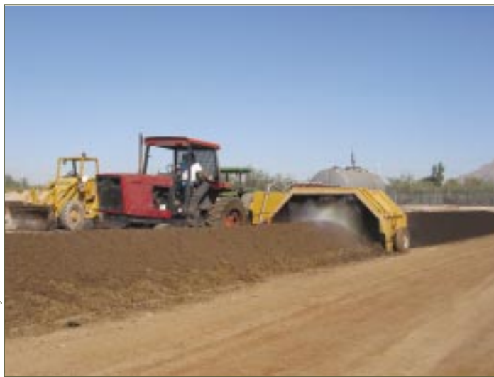
As a part of the composting process, this tractor attachment turns, waters and aerates the manure pile.
