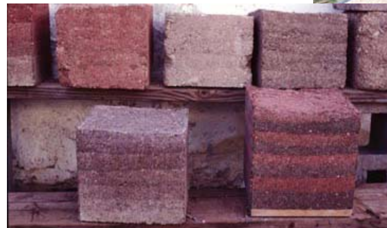
Experimental blocks of rammed earth with color additives.
