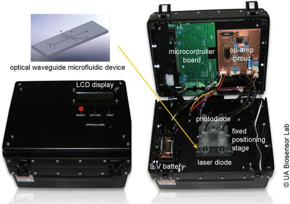
First prototype of lab-on-a-chip system for detecting microbes in water, food and air
