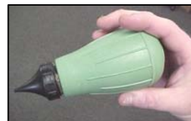
A bulb duster is used to apply DE into cracks and crevices
